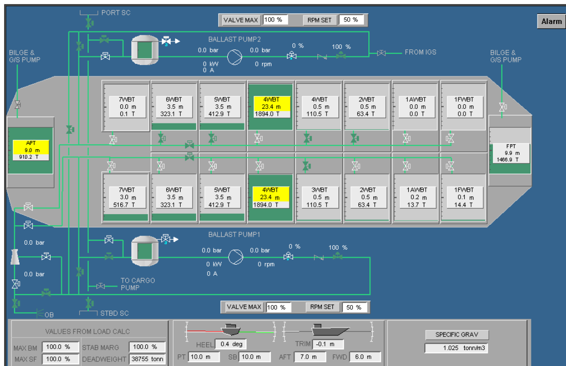
Figure 83 Typical Ballast Process image
