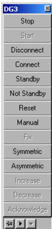
Figure 59 Generator control operation menu extended
