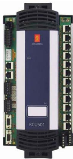
Remote Controller Unit (RCU) is a real-time single board computer and remote IO bus driver
