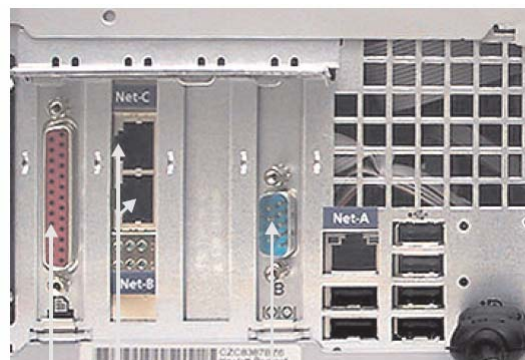
Parallel port Network card NET C (above) NET B (below) Serial port (COM2)
