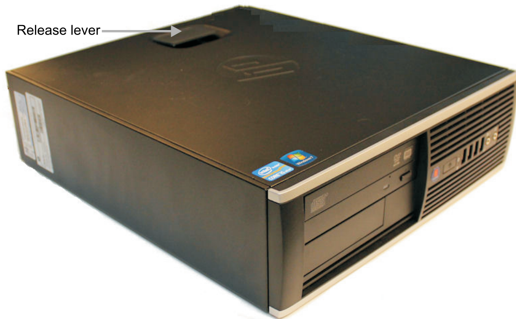
Figure 8 Release lever of the cabinet lid
