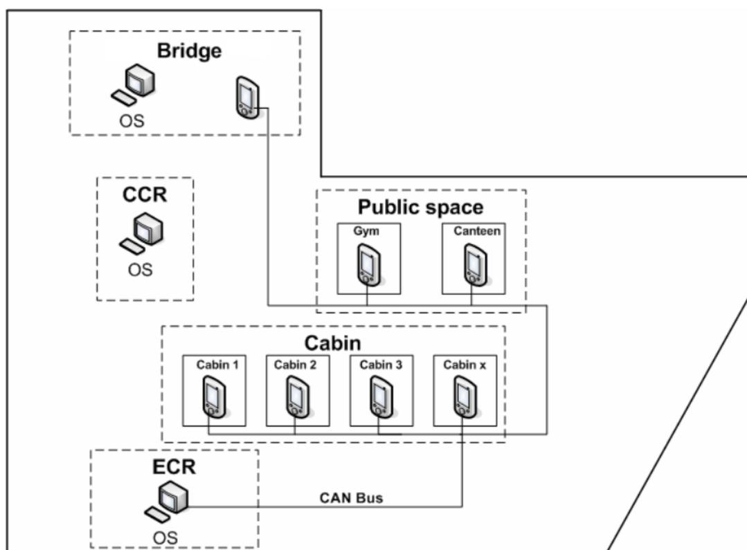
The main purpose of the WCS is to allow critical locations such as the Engine Control Room (ECR) to be temporarily operated unmanned (during night shift or during loading/off-loading etc). In addition to Engine alarms, alarms from other spaces such as the Cargo Control Room (CCR) can be integrated as autonomous parts of the WCS. Some definitions of the main concepts in the WCS are explained in the table below.
