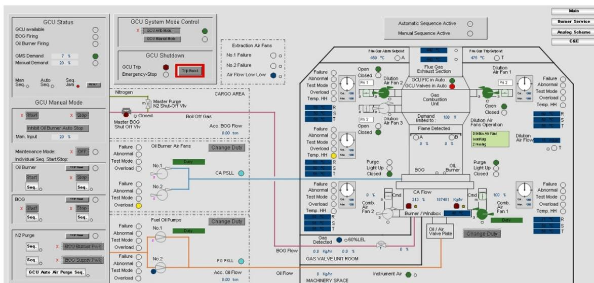
The GCU operation panel contains buttons of control of sequences and lamps for feedback.
