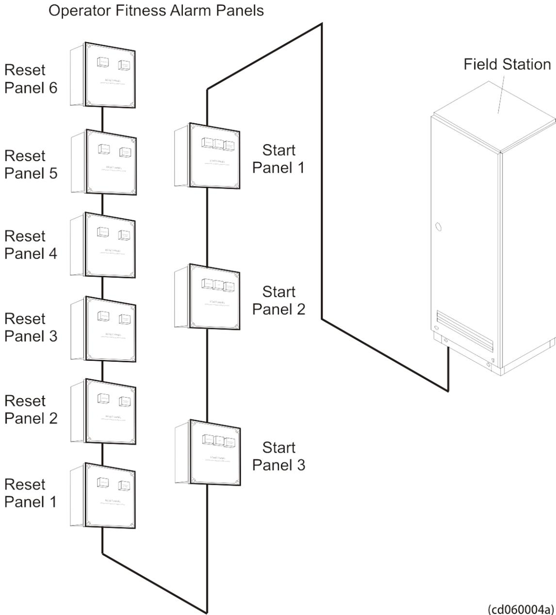
The Start Panel, located in the entrance of the Engine Room, is connected by a single cable to a Remote Controller Unit (RCU) in a Field Station (FS) in one end and to the Reset panels in the other end. The FS is further connected by the local area network (LAN) to the K-Chief 700 OS from which the OFAS status can be remotely observed.
