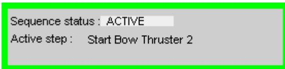
An example of a typical Sequence process view for a Vessel Control mode transfer is shown in the figure below.
