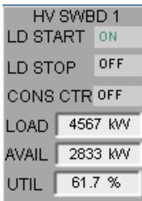
You can turn the **Load Start**, **Load Stop** and **Consumer Control** on or off from the module operation menu. To open this menu, use the left trackball button to click the **ON/OFF** label in the **Load and Consumer Control** status field.
