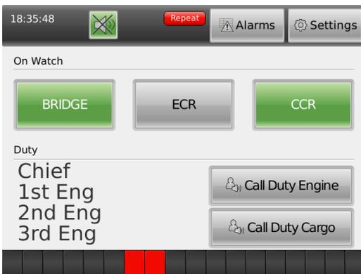
A flashing indicator will appear in the bridge unit top bar when there is a repeated alarm
