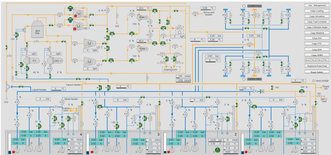
From the Cargo-Plant Process image you can monitor the deck piping instruments (sensors for pressure, temperature and flow) and valve position indicators. Temperature pressure sensors in void spaces are interfaced to the K-Chief 700 by means of barriers installed in the Process Stations.
