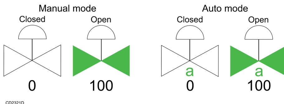
Figure 44 On/off valve module symbols
