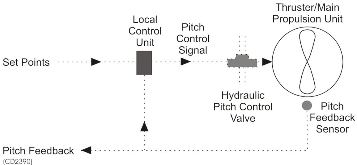
Local (non follow-up) control is normally achieved by means of control handles on the local hydraulic-pitch valve control unit or tailor-made control panels interfaced to the hydraulic-pitch valve control unit.
