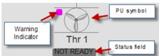
The state of each PU is indicated by the color of the PU symbol, the text and the background color in the status field adjacent to the PU symbol and a warning indicator as listed in the tables below.
