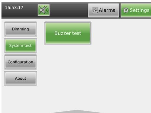
Pressing the **System Test** button displays a test window. A **Buzzer test** button lets the user test the alarm sound. Pressing the button again turns the test off. The user also has the option to use the “Sound Off” soft-button appearing in the top bar :
