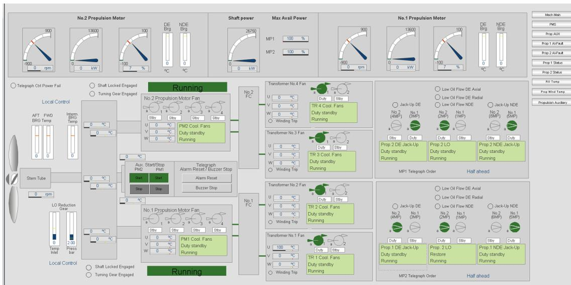
For an electrically driven main propulsion unit, the motor together with bearing, temperature and winding temperature measurements, and pump and cooling fan status may be shown.
