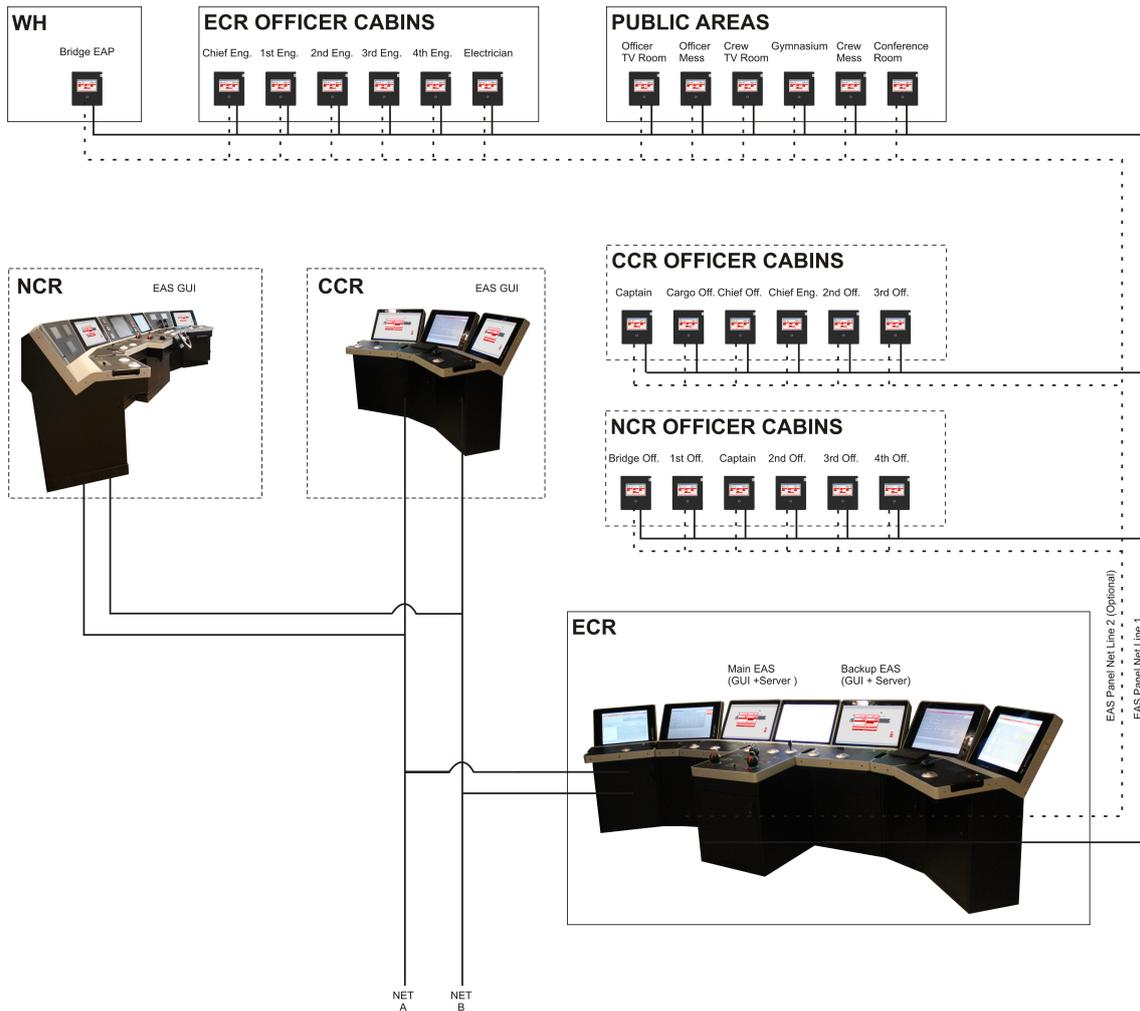
The main purpose of the EAS is to allow locations such as the *Engine Control Room (ECR)* to be temporarily operated unmanned (during night shift or during loading/off-loading etc). In addition to Engine alarms, alarms from other spaces such as the *Cargo Control Room (CCR)* and the *Navigation Control Room (NCR)* can be integrated as autonomous parts of the EAS.
