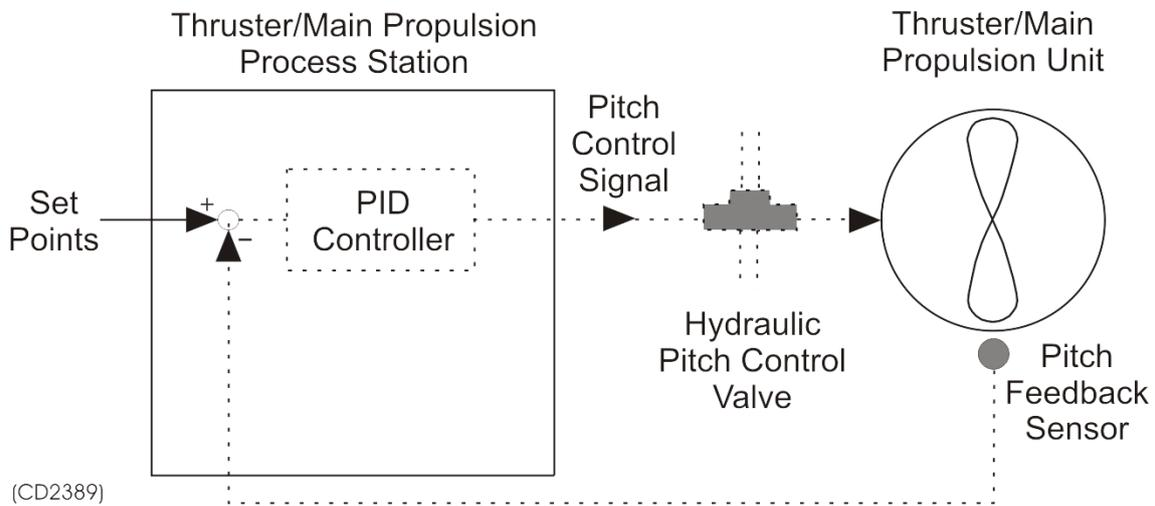
Manual pitch control, which is implemented by means of the commands on the PID controller module operation menu, is only possible in the **Maintenance** mode. See the section *Maintenance mode* on page 113 and the section *Typical procedures* on page 114.
