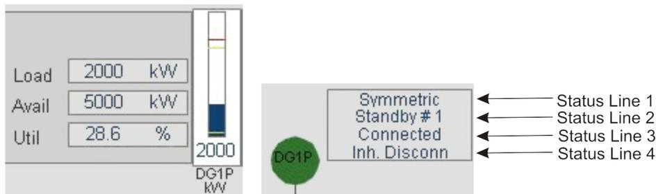
Optional information such as the power factor, output voltage, load current and frequency of the generator can also be shown near the generator symbol.
