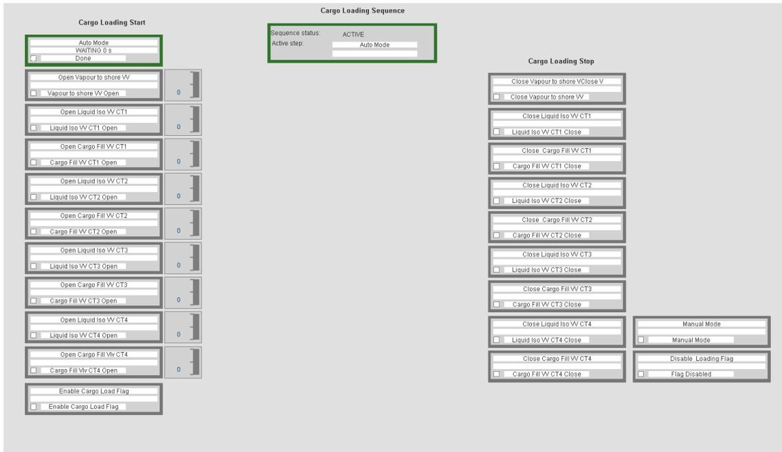
Figure 54 Sequence process image for cargo loading - detail
