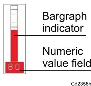
The colour of a bar graph indicator and the background colour of the numeric value box.
