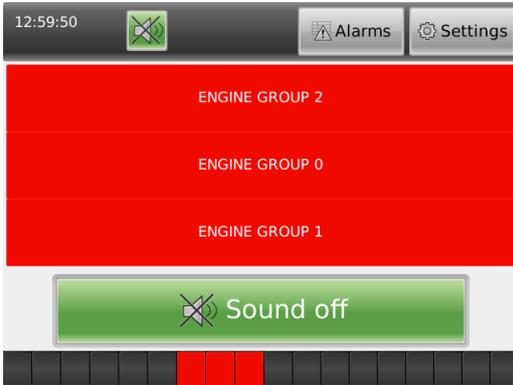
When an alarm condition occurs the buzzer will sound and the alarm is indicated on the Watch Cabin Unit.
