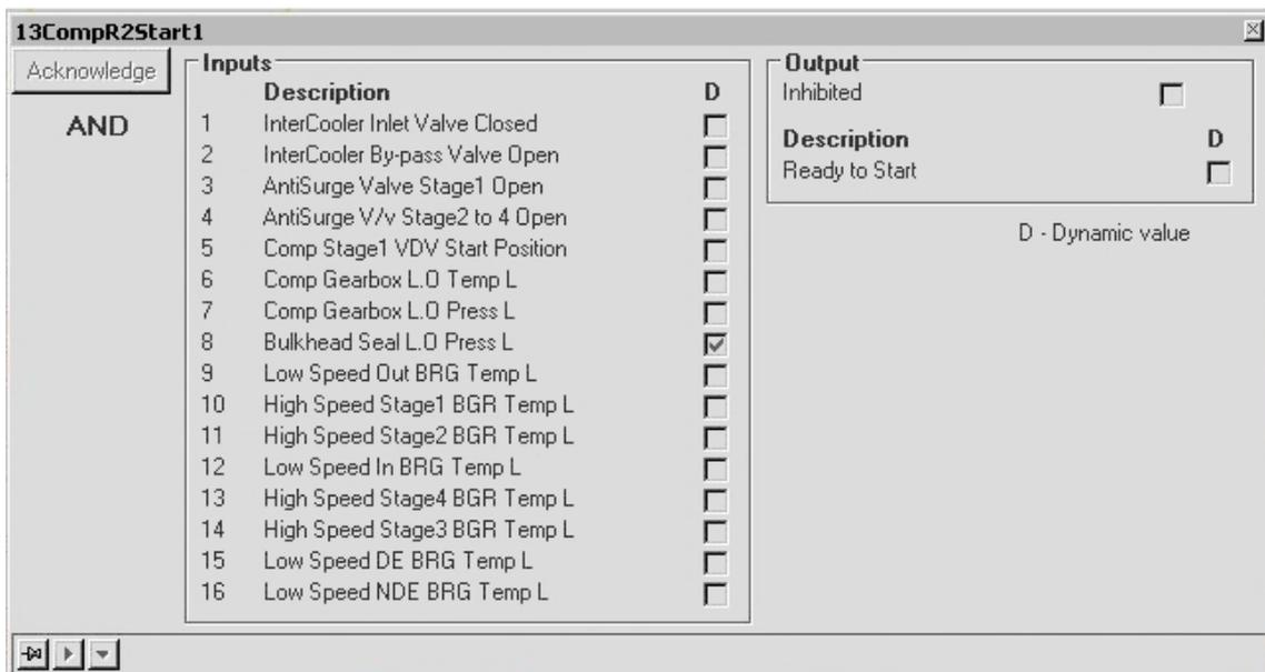
In the pop-up window all interlock criteria will be displayed with description and the criteria states will be indicated by a mark in the **D (Dyanmic)** column.
