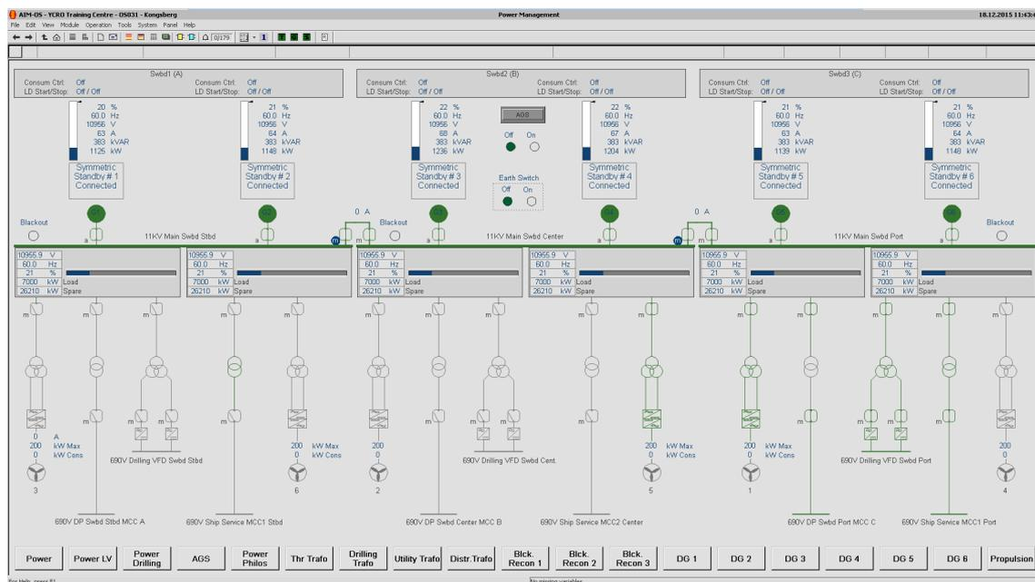
You can view some of the equipment in more detail by selecting a lower-level process image. The contents of the lower-level process images depends on the equipment installed on the vessel. For specific information on a device, see the user documentation for the device. For example, you can click the DG1 button at the right of the top-level power management screen to view the generator set process image for diesel generator 1.
