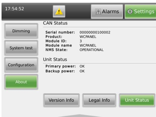
The Top Field of the panel contains additional information. A digital clock is localized in the upper left field. A warning signal and a failure warning button appear if the system has an error condition.
