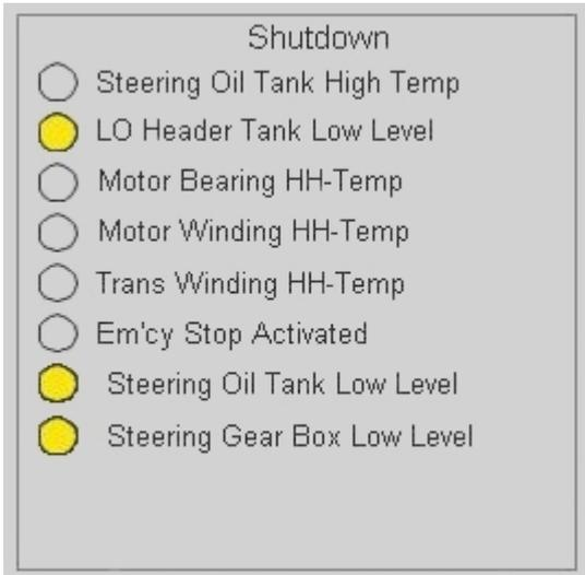
A digital measurement module can also be shown as a symbol that changes colour to give the status. See the section *Process status indication* on page 40.
