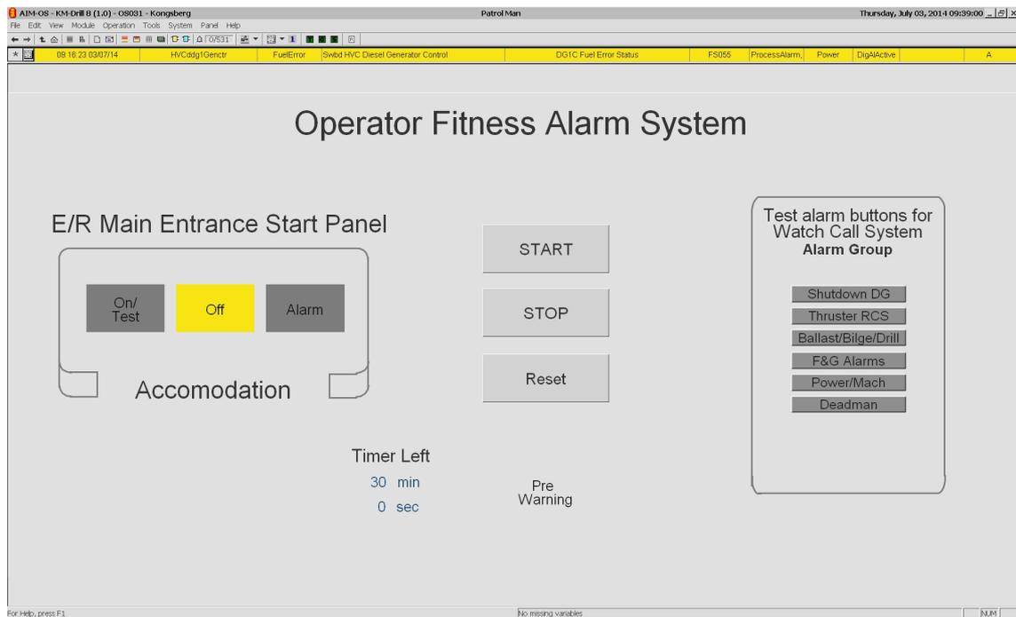
The Reset period is set to 30 minutes and a pre-warning alarm is given 5 minutes before the operator fitness/dead man alarm is initiated. If an active OFAS is not manually turned OFF or reset within the specified reset period, the OFAS/ Dead Man alarm is shown in the **Event List** on the K-Chief OSs and on the EAS/Watch Call Panels.
