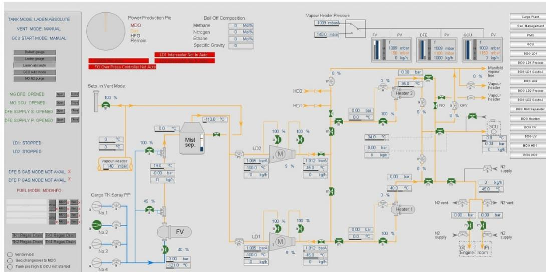
The Gas Management System will try to keep the cargo tank pressure within normal operation limits. It also includes safety function if the tank pressure exceeds the normal operation limits.
