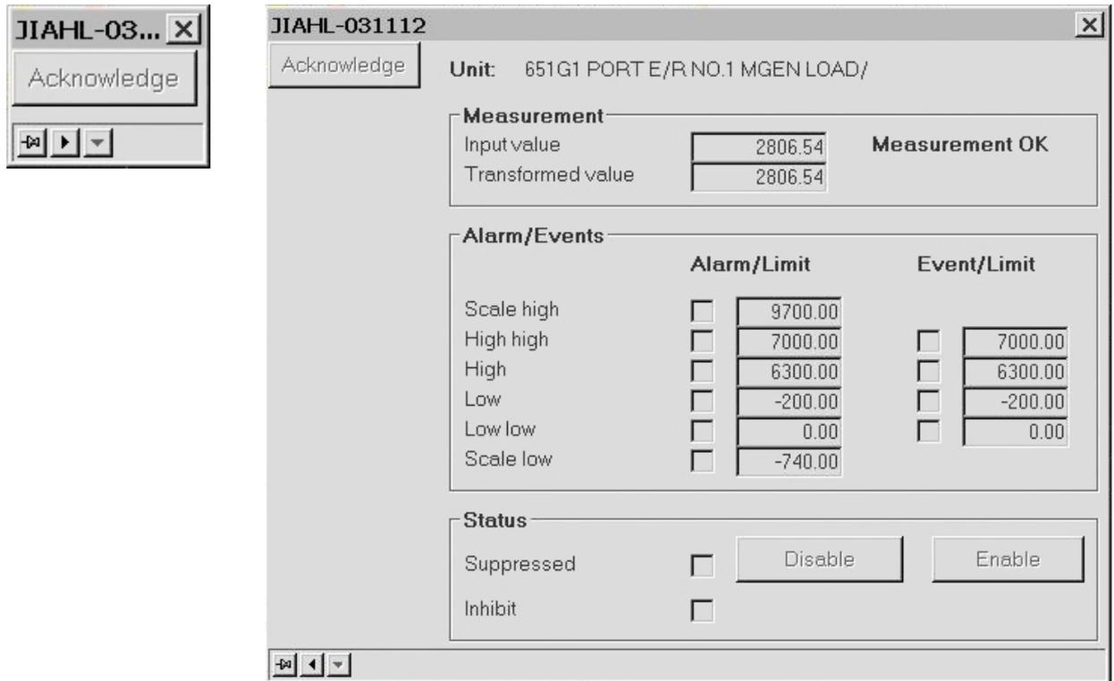
Click the command buttons to **Enable** or **Disable** the alarm suppression function. When you disable the alarm suppression, it is automatically enabled again after 10 minutes.
