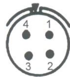
Fig. 11-5: Pin Lay-out and Pin Assignment Peripheral Socket
