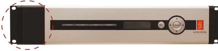
When the Power/SW LED turns green, the unit is running.
