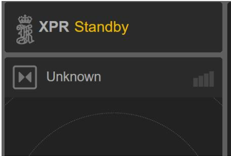
If the XPR system is set to **Automatic** target selection and a target is selected on the dynamic positioning (DP) system, the DP sends a target selection telegram to the XPR. If this target does not exist in the XPR system, a new target will be created. This new target contains only the correct **Id** and location (**Latitude/Longitude**), all the other parameters have to be entered.
