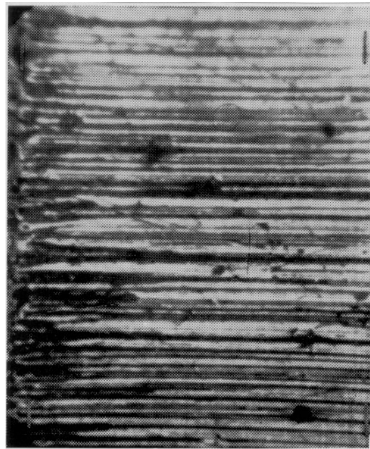
Photo 1 (X30) Rough scratching (degree 5) of a top piston ring running face. The photo shows the upper edge, where the hard particles enter between ring and liner wall. This scratching is quite fresh, i.e. recovery or restoration has not yet commenced. Designation S5NEW.
