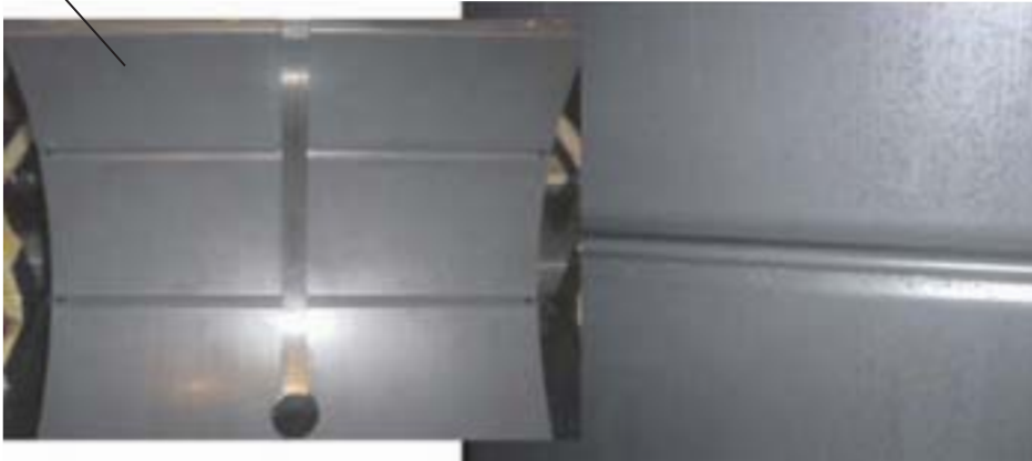
Fig. 63: Synthetic overlay on AlSn40 crosshead bearing shell
