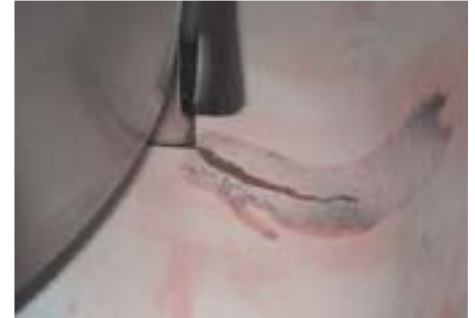
Fig. 66: Crack in camshaft bearing pedestal
