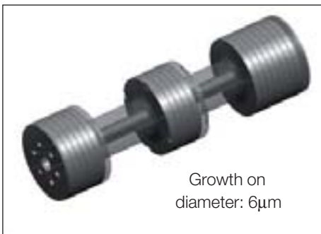
Fig. 22: FIVA valve, growth of main spool
