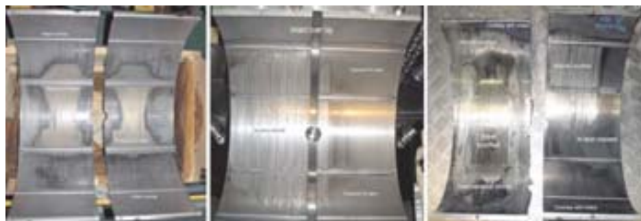
Partially corroded overlay, not yet scuffed
