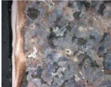
Fig. 53: Piston ring with 'white layer'
