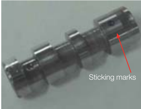
Fig. 17: ELVA valve, sticking high- response valve spool
