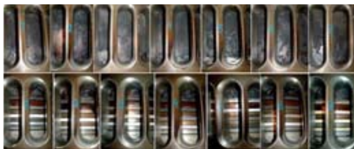
Fig. 11: 7S50ME-C, cylinder condition after 10,717 running hours
