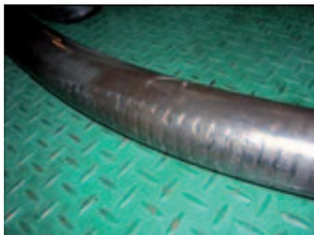
Fig. 28: Exhaust valve high pressure pipe: Serious dent marks has been observed
