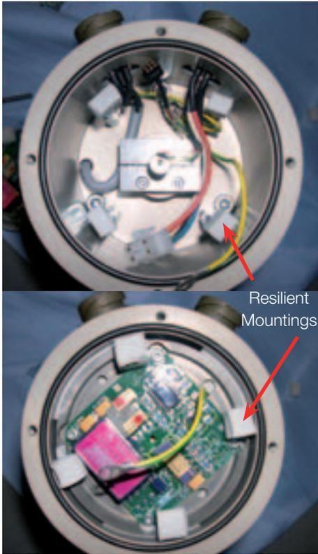
Fig. 13: ELFI valve, PCB secured by resilient mountings
