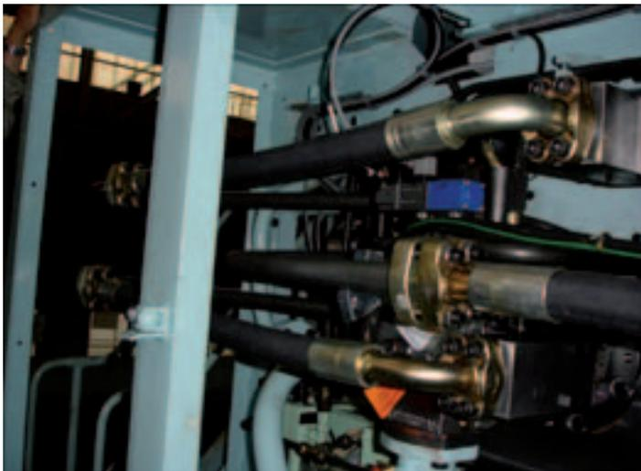
Fig. 33: Flexible hoses on K98
