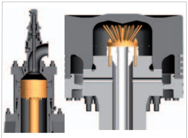
Fig. 53: Piston cooling insert
