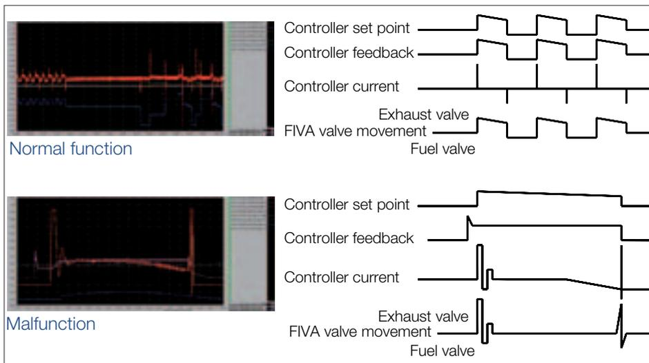
Fig. 21: Uncontrolled feedback signal due thermal overload of FIVA electronics FIVA valve, growth of main spool
