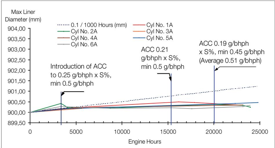
Fig. 46: Cylinder liner wear, cylinder oil reduction test, 6S90MC-C (M/T Astro Cygnus)
