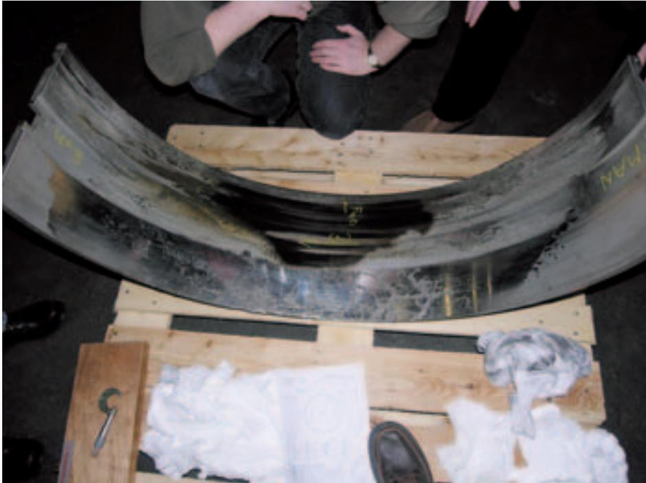
*Fig. 62: K98MC-C, crankpin bearing upper shell damaged by foreign material entered through the oil way*
