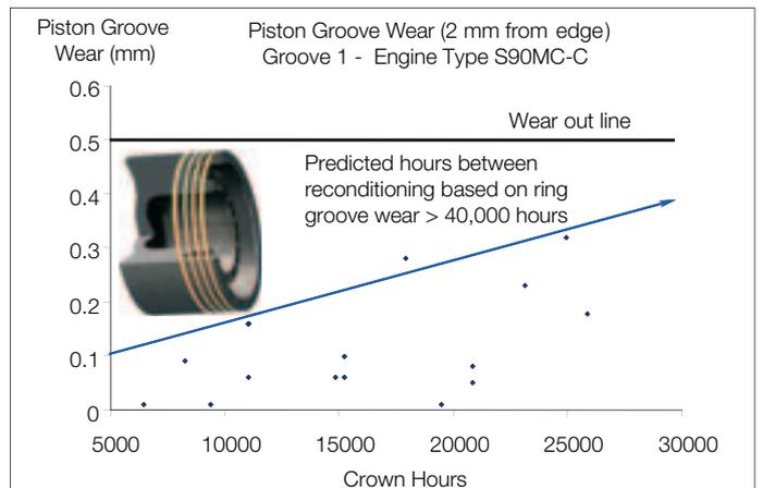
Fig. 49: 6S90MC-C, Piston ring groove wear
