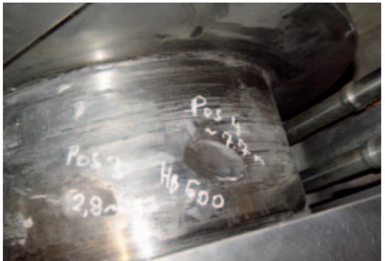
Fig. 60: Main bearing journal as result of steel-to-steel contact
