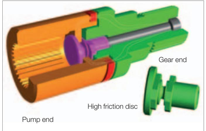
Fig.35: Pump safety shaft, new shaft assembly with central bolt
