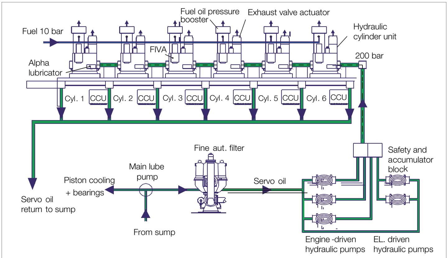
Fig. 8: Hydraulic loop of the ME engines
