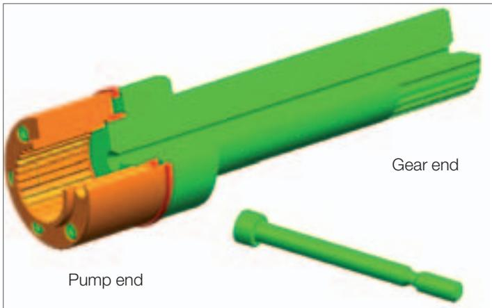
Fig. 34: Pump safety shaft, initial design
