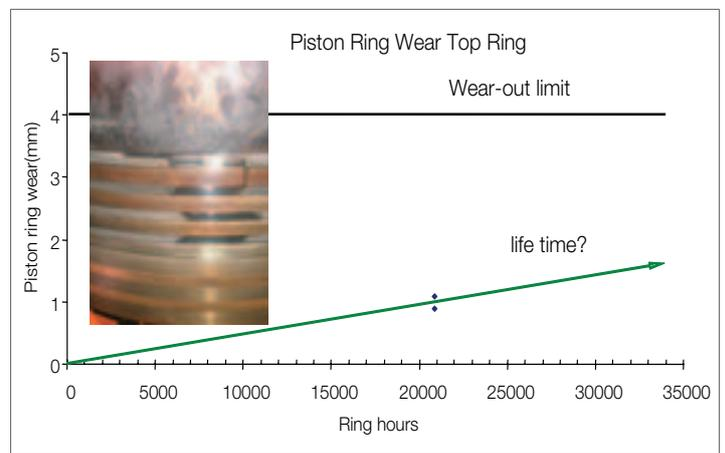
Fig. 45: Piston ring wear measurements, 6S90MC-C (M/T Kos)
