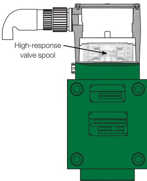
Fig. 14: ELVA valve, location and high-response valve spool
