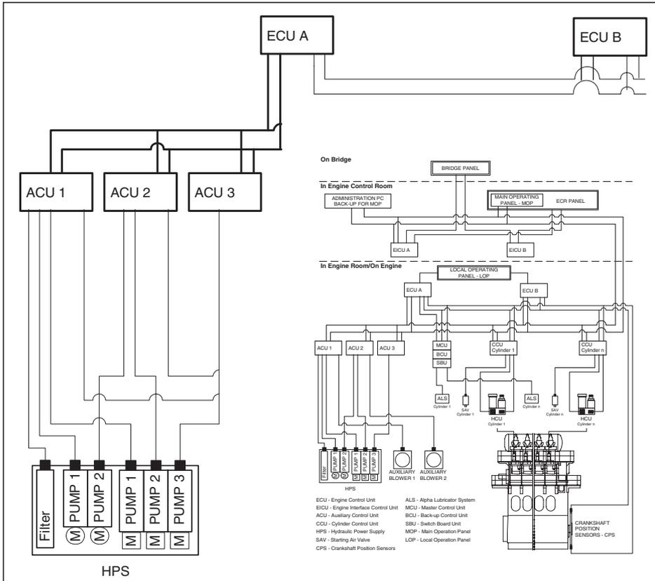
Fig. 40: ME-system, control diagram (initial version)
