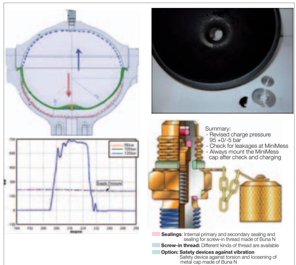
Fig. 25: Maintenance of accumulators
