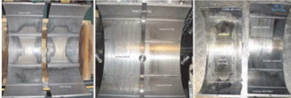
Partially corroded overlay, not yet scuffed
