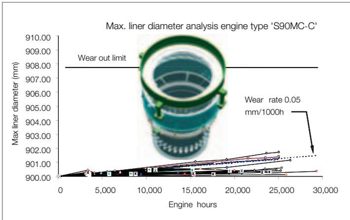
Fig. 47: 6S90MC-C, cylinder liner wear
