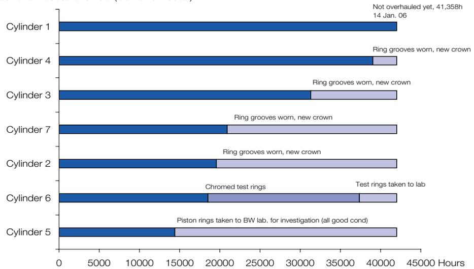
Fig. 54: 7K98MC, condition-based overhaul piston No. 1 overhauled first time after 42,500 hrs
