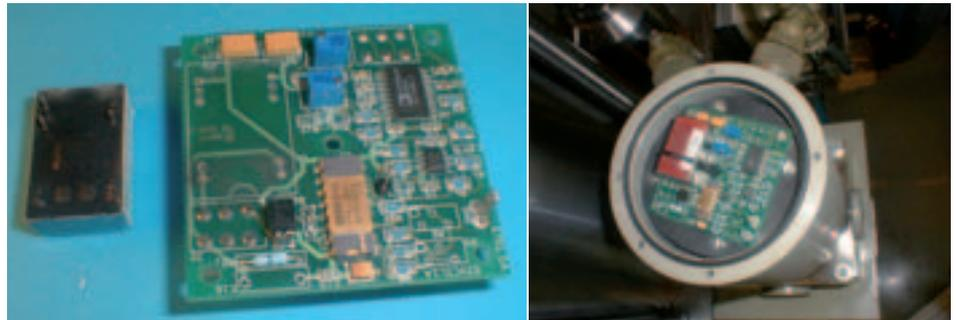
Fig. 12 : ELFI valve, DC-DC converter coming off due to vibration of PCB
