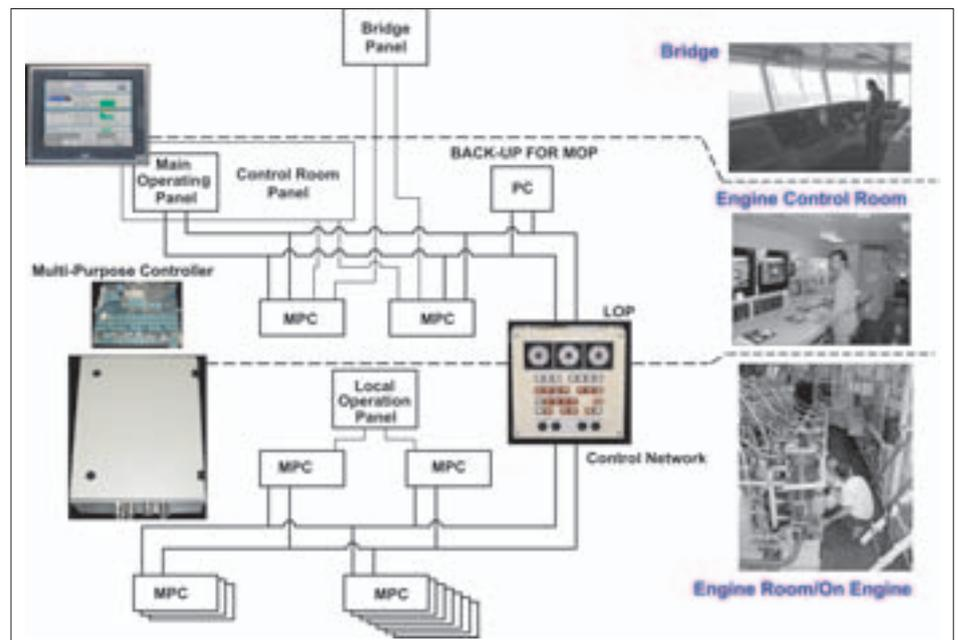
Fig. 7: Engine Control System (ECS)
