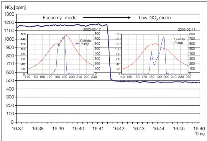
Fig. 3: Flexibility with respect to emission
