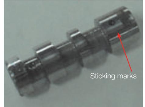
Fig. 15: ELVA valve, sticking high-response valve spool
