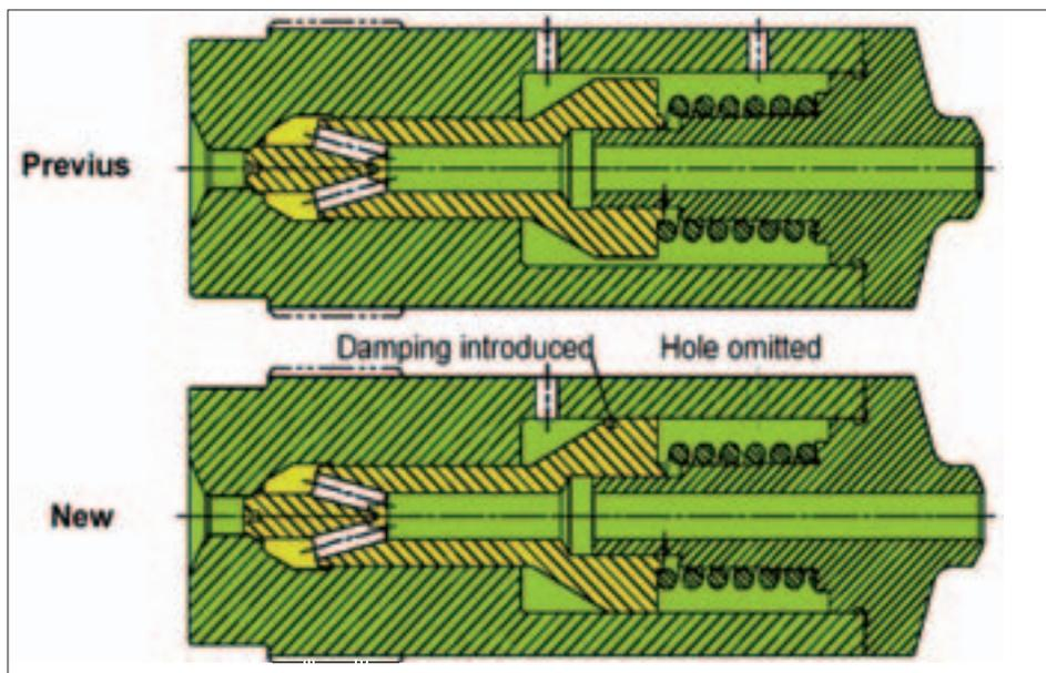
Fig. 27: ME-fuel injector: internal damping applied at non-return valve
