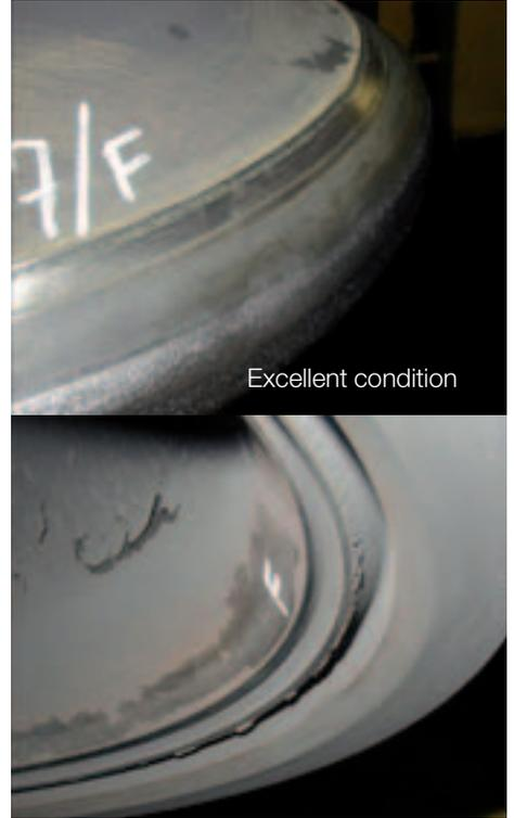
Fig. 50: Nimonic exhaust spindle and W-seat bottom piece
