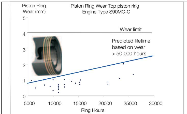
Fig. 48: 6S90MC-C, Piston ring wear
