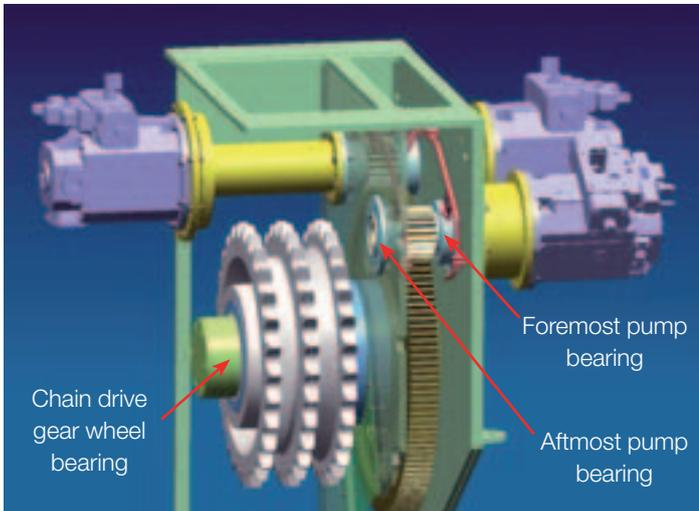
Fig. 30: HPS gearbox: Position of bushings
