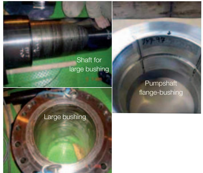
Fig. 31: HPS gearbox: Failed bushings/bearings
