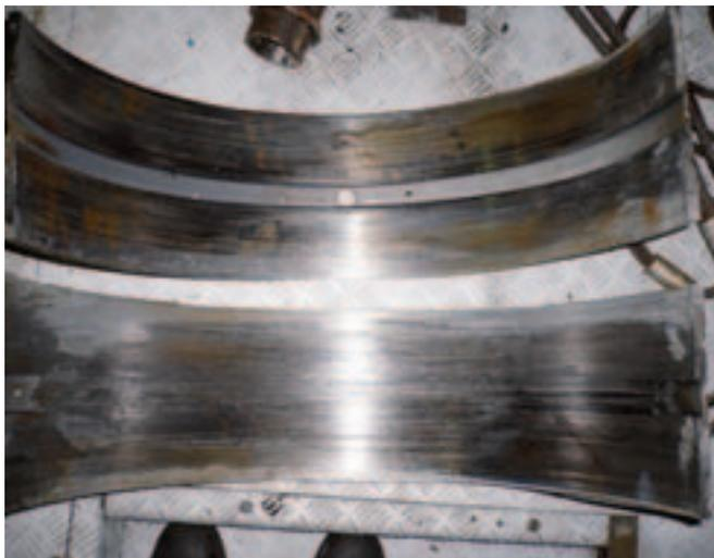
Fig. 59: Steel-to-steel contact in thin shell main bearing shells
