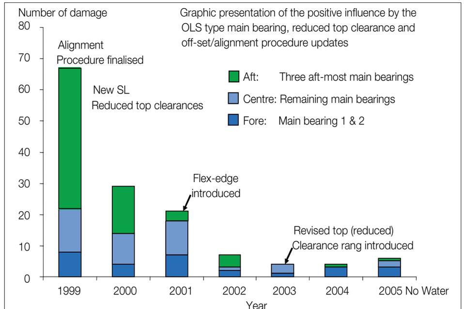
Fig. 55: Main bearing damage statistic
