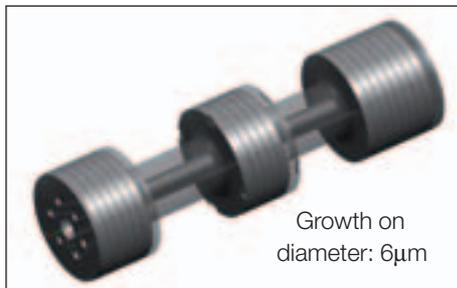
Fig. 20: FIVA valve, growth of main spool
