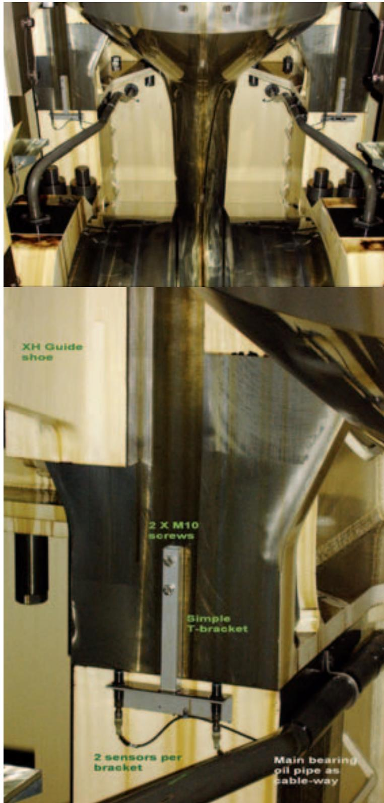
Fig. 61: BWM installation on a K98MC-C
