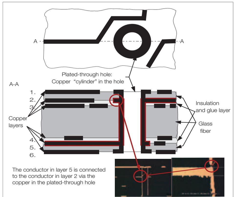
Fig. 38: PCB, broken copper layers
