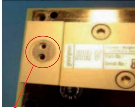
The spring force in the connector has disappeared due to sparks/high temperature
