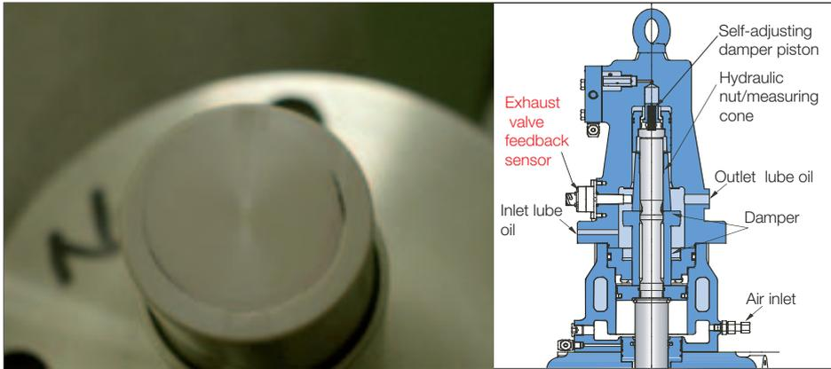
Fig. 23: Exhaust valve feedback sensor
