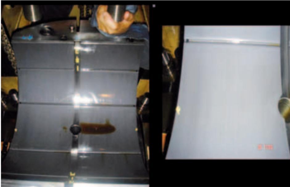
Fig. 58: Synthetic overlay on AlSn40 crosshead bearing shell after 10,000 hours
