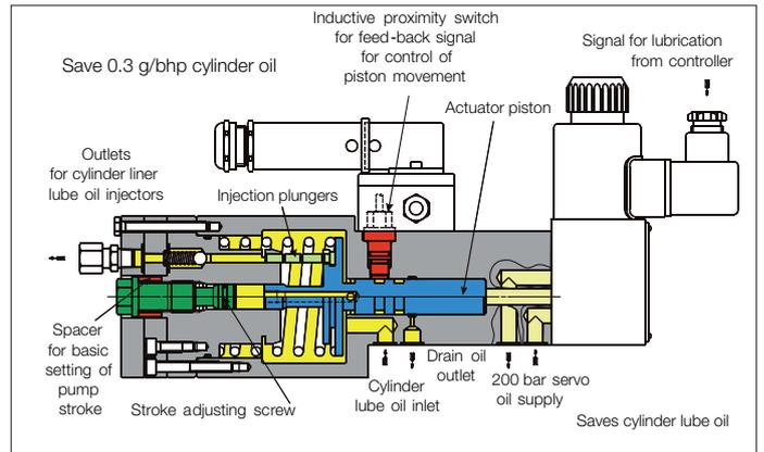
Fig. 5b: System integration, example: Alpha Lubricator
