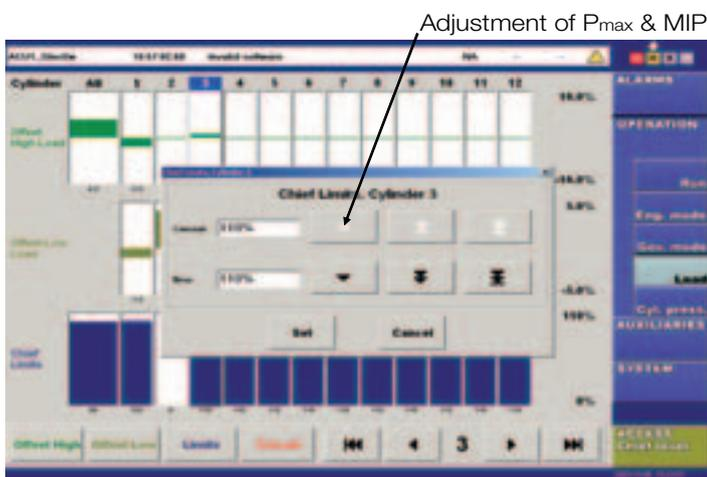
Fig. 4: Easy engine balancing/adjustability
