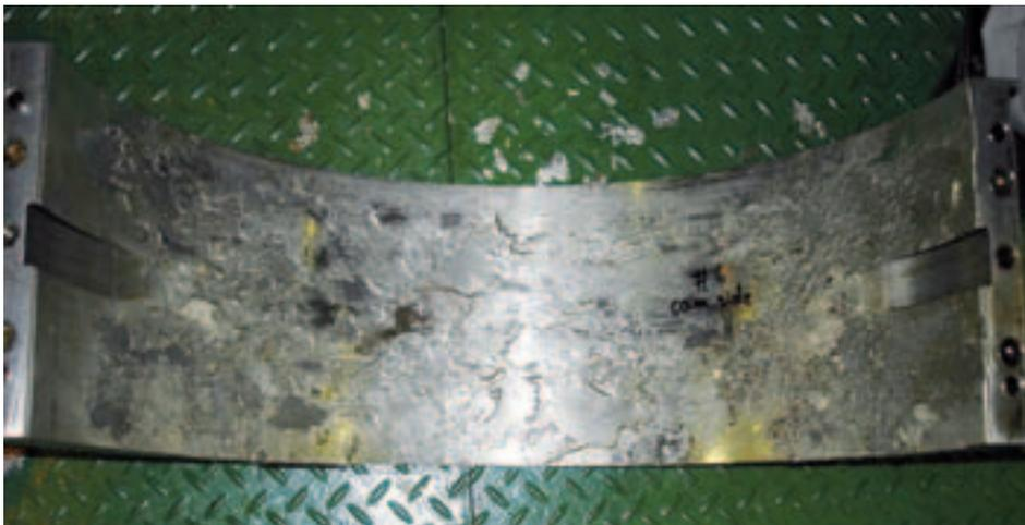
*Fig. 63: Thick shell main bearing severely, but not yet critically, damaged. Bearing lining worn, but not yet worn away*
