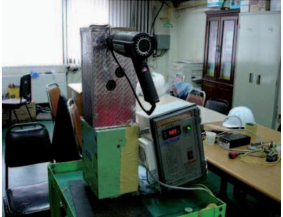
Fig. 22: Temperature test of FIVA valve with mobile equipment, the valve is connected to a CCU during the test
