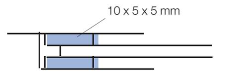
Fig. 18: FIVA valve, resilient mounting of PCB
