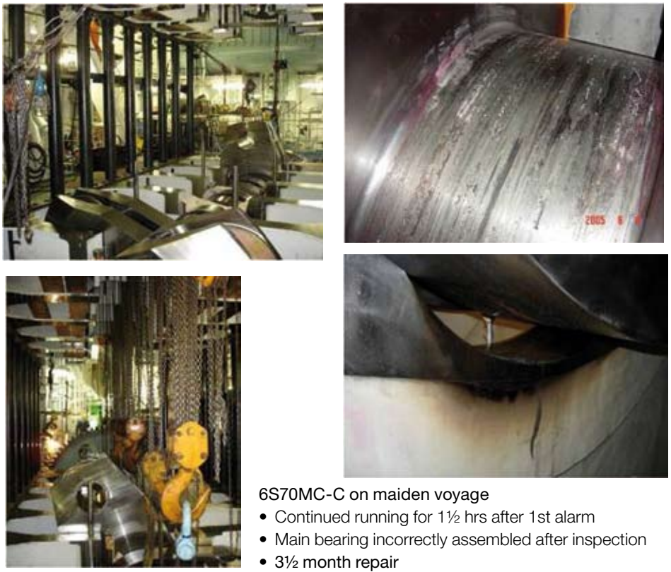
Fig. 8.37: Main bearing damage on 6S70MC-C
