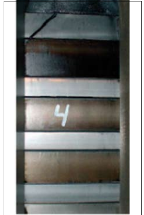
Fig. 8.30: Unit running very well after 20,021 running hours. Note that the last remains of the alu-coat are still visible on the lower edge, indicating remaining rounding left. This means that the ring wear is less than 2 mm out of possible 3 mm. Consequently, many more hours are left from the point of view of wear.
