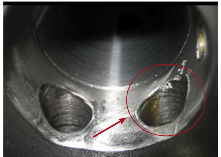
Fig. 8.11b: Cavitation in exhaust actuator top cover
