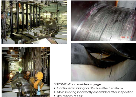
Figure 45 – Main bearing damage on 6S70MC-C
