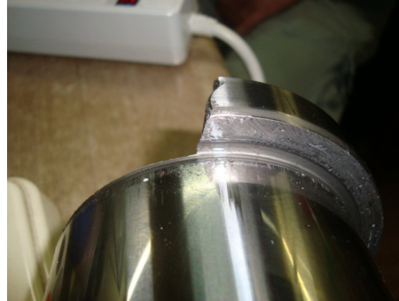
Figure 4 – Piston collar breakage
