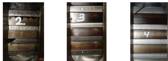
Figure 36 – (2) Totally scuffed unit. Lubrication should be increased to maximum until overhaul is convenient with regard to the schedule of the ship. Due to the friction heat developed, the piston rings get hardened, and the wear rate of the liner increases significantly. However, the hardening protects the rings, which is why operation may be continued safely until next convenient port stay.
