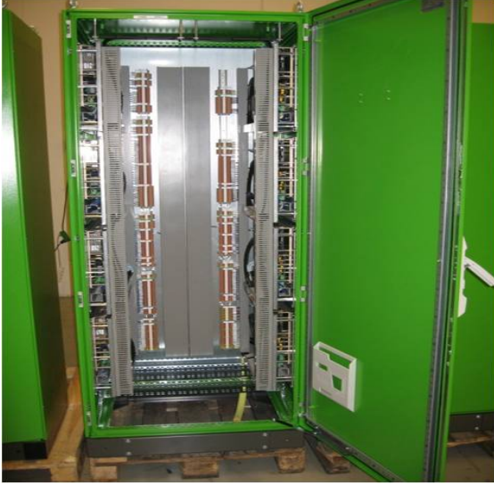
Figure 13 – Large cabinet suited for engine control room placement
