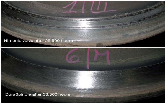
Figure 40 – W-seat in combination with nimonic spindle and DuraSpindle
