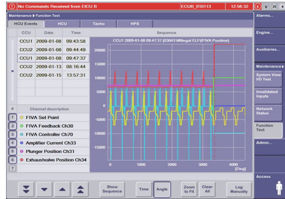
Figure 11 – New ECS software with trouble shooting screens
