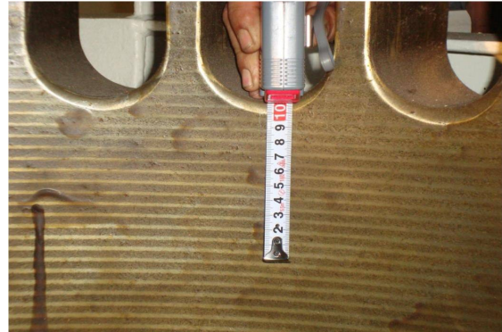
Figure 21 – Cylinder liner quality: insufficient plateau honing
