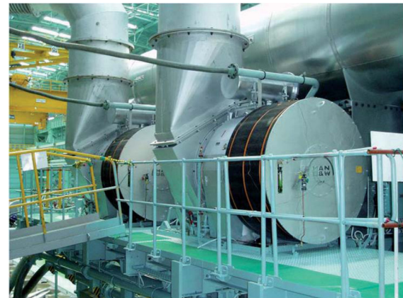
Figure 47 – Modern turbocharger enabling more than 30,000 hours between major overhauls
