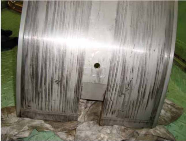
Fig. 22: Upper main bearing shell backside
