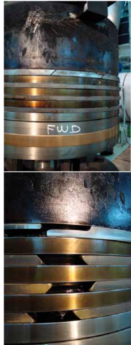
Fig. 26: ME-B9 piston after 4,000 hrs
