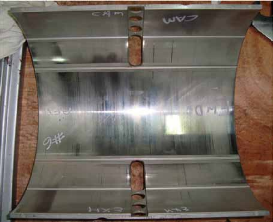
Fig. 28: ME-B9 crosshead bearing after 4,000 hrs.
