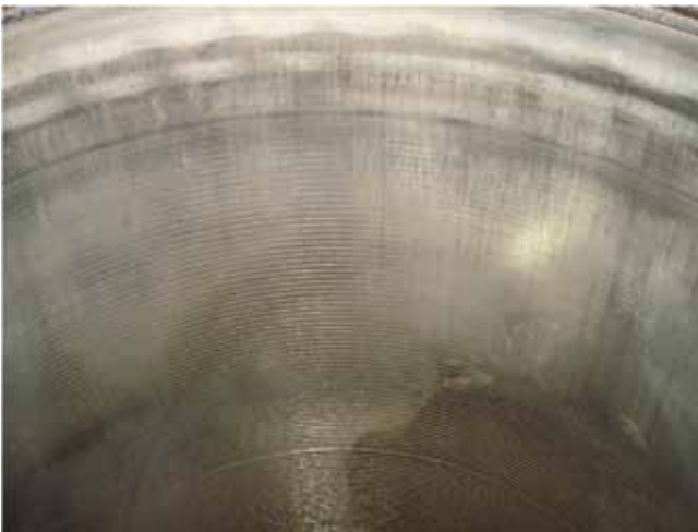
Fig. 18: Top of liner after 3,800 hrs.
