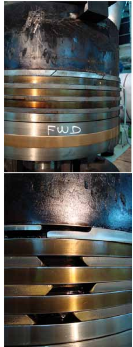
Fig. 26: ME-B9 piston after 4,000 hrs
