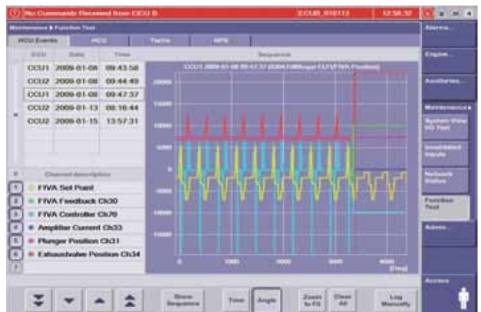
Fig. 11: New ECS software with trouble shooting screens: HCU event recorder
