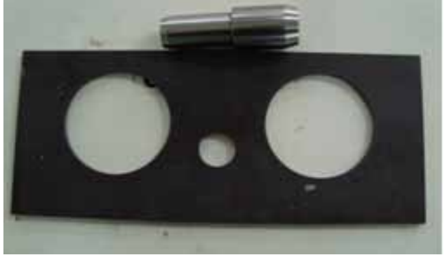
Fig. 20: High-friction shim and guide pin
