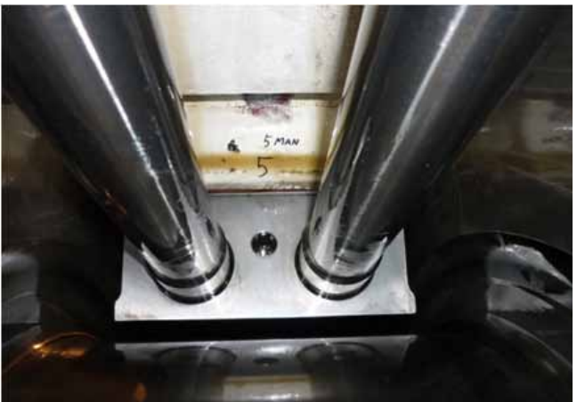
Fig. 21: Main bearing cap and bedplate contact area
