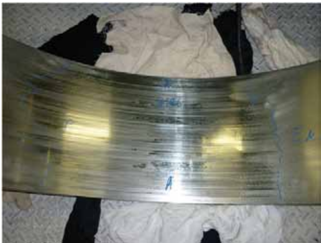
Fig. 23: Lower and upper shell, white-metal side
