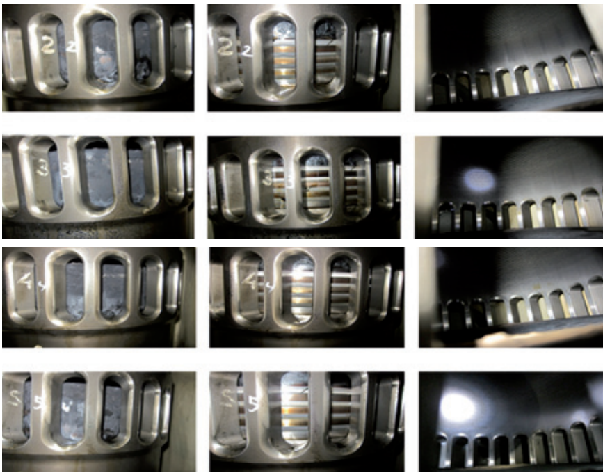
Fig. 20: Scavenge port inspection of prototype 6S40ME-B at 10,000 hours
