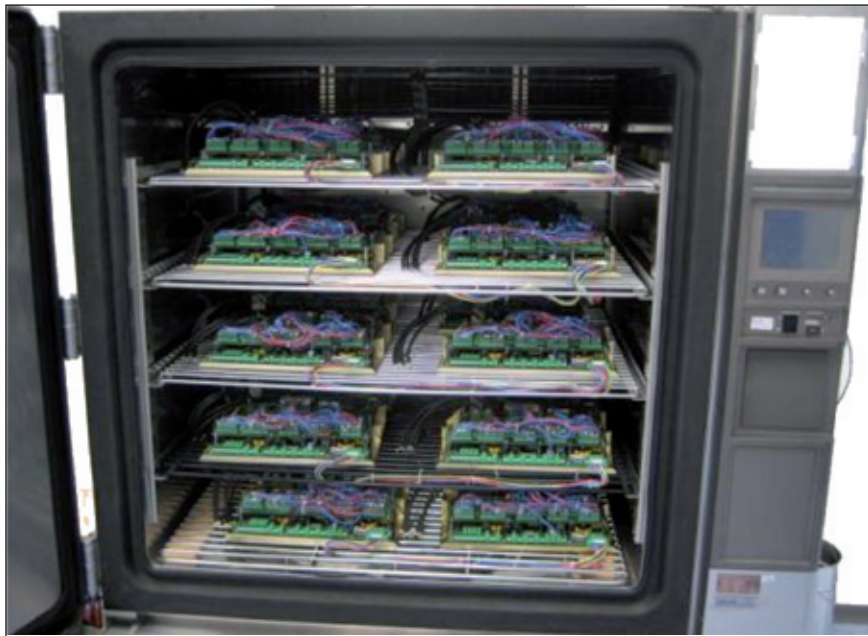
Fig. 1: Burn-in test of MPCs
