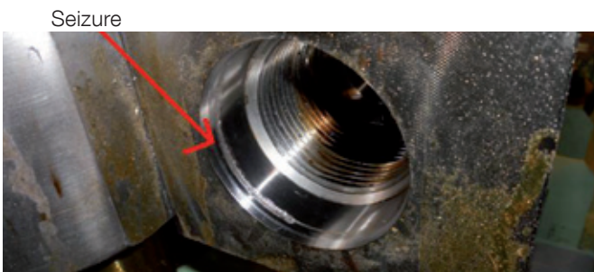
Fig. 35: Seizures on distributor block and pipe union
