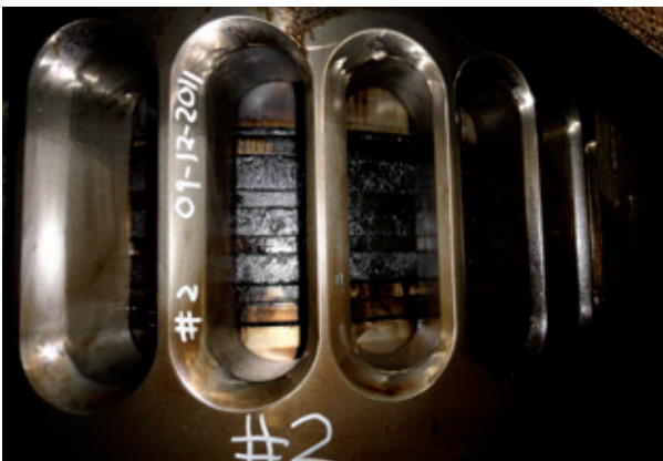
Fig. 28: S80ME-C9: Collapsed/broken piston rings
