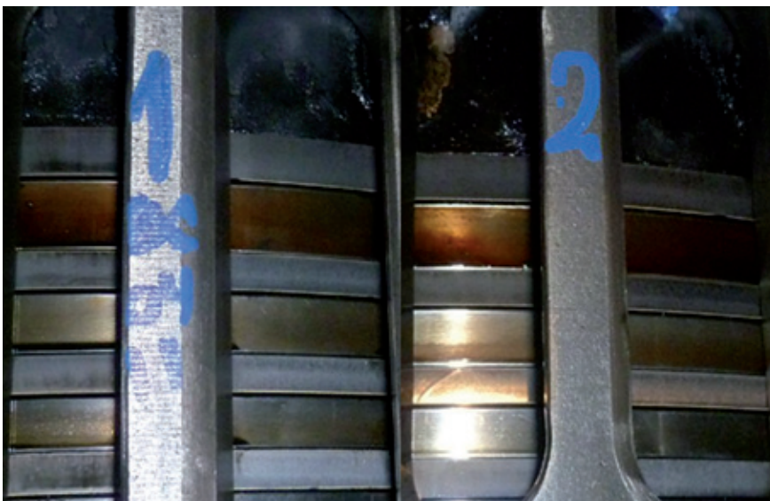
Fig. 23: 6S46MC-C unit with POP ring pack
