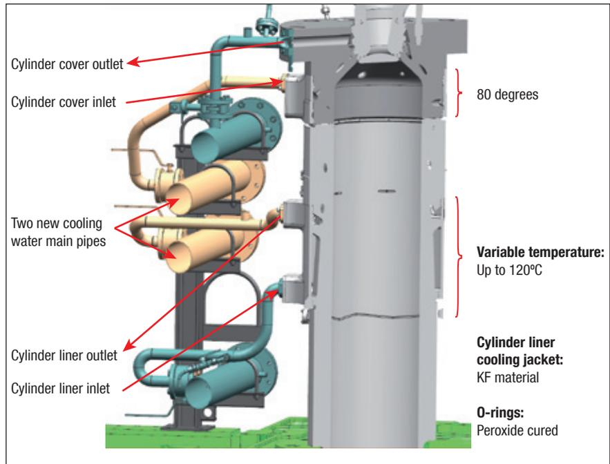
Fig. 31: Controlling corrosive wear: 4-pipe jacket cooling water system
