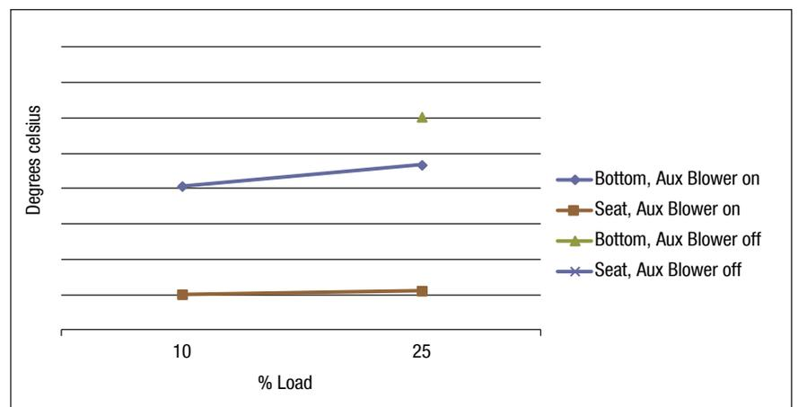
Fig. 25: Influence of auxiliary blower cut-in during low-load operation on a 10S90MC-C9.2
