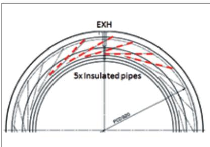
Fig. 28: S70 semi-high topland: insulated cooling pipes
