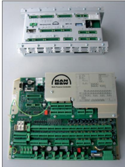
Fig. 1: MPC10 (upper) and MPC (lower)
