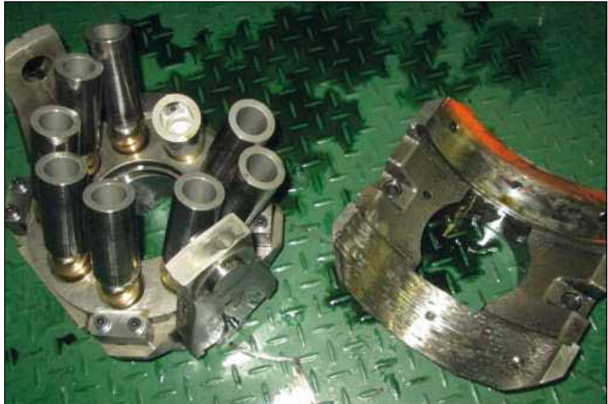
Fig. 57: ME engine Eaton main hydraulic pumps. Pump swash plate/piston assembly, bearings and holder damaged
