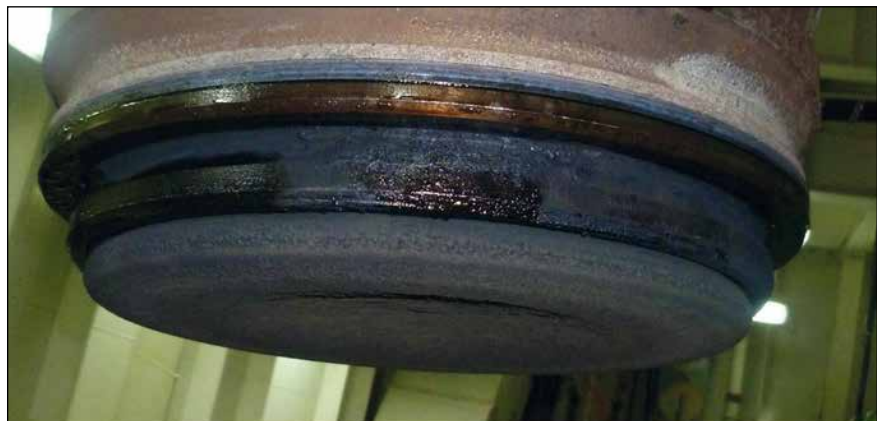
S60MC-C8: Running hour 26,000 Burn away: >11 mm (max. 9 mm)
