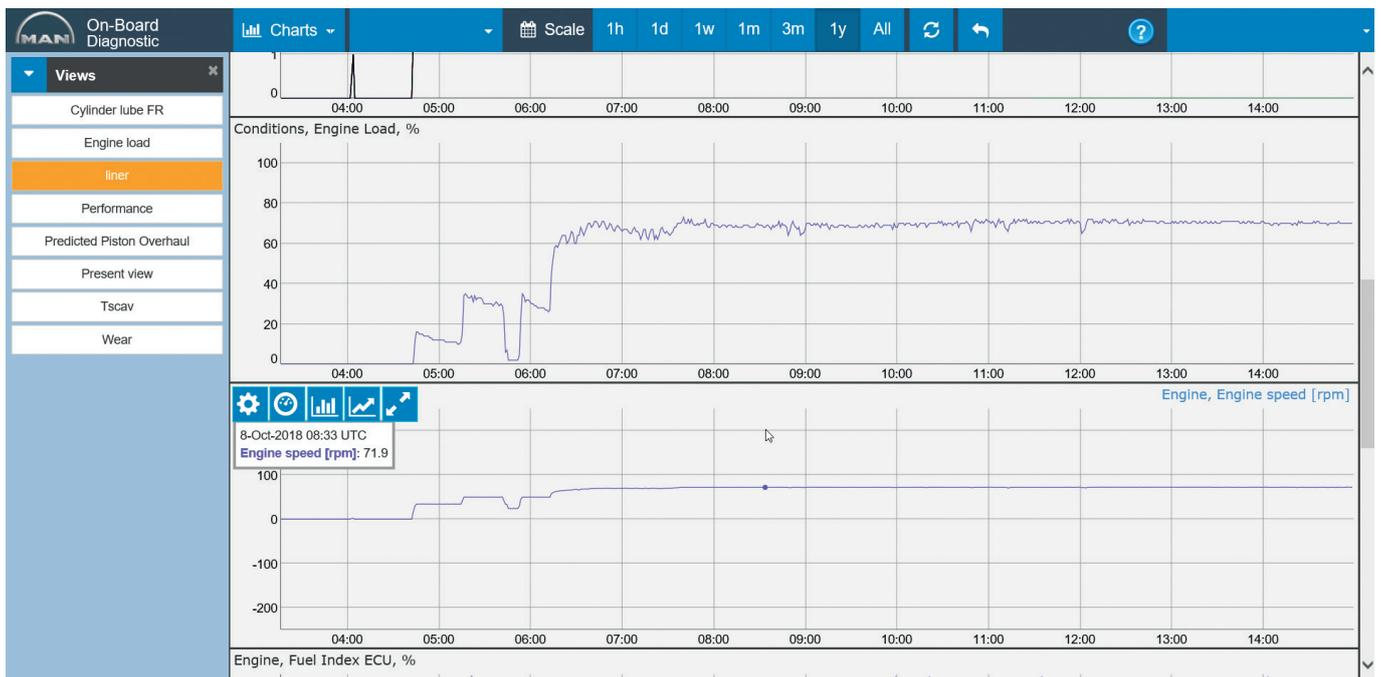
Fig. 48: Engine rpm and load from the OBD
