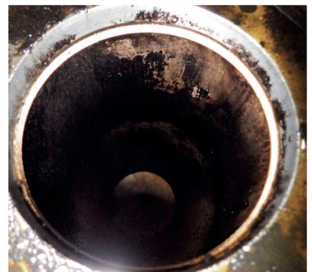
Fig. 63: Coke deposit in the spindle guide
