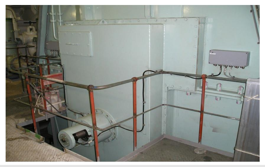
Tacho system – Trigger ring and sensors (option)
