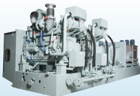
Hydraulic power unit with a combination of electric motor driven power packs and diesel engine driven power packs for medium and large sized tankers.
