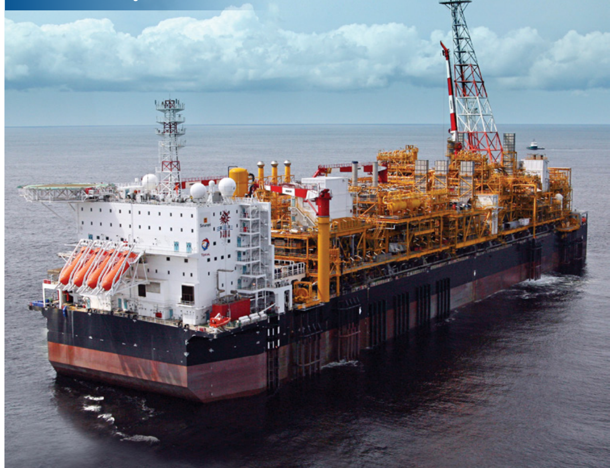
FPSO "DALIA" 2 mill bbls for Elf Exploration Angola (Total). Built Samsung Heavy Industries, Korea. Service at Dalia field in Angola since 2006.
