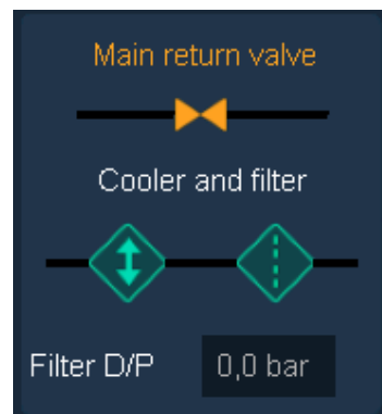
Override state on Main return valve
