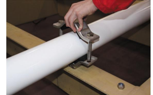
Remove the bolts, and lift of the upper steel body part. The lower part is welded to the structure.
