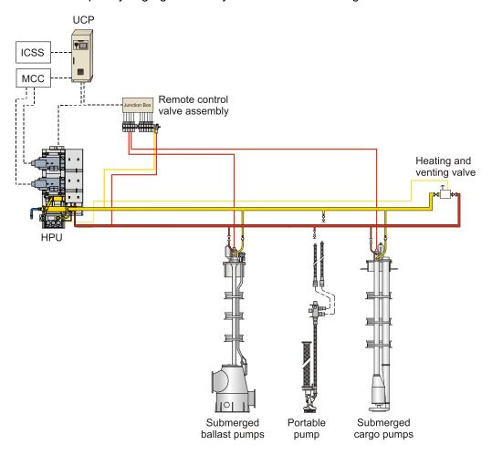
The hydraulic power unit consists of electric motor driven hydraulic power packs, where the hydraulic pumps are of axial piston type and swash plate design with variable displacement. The pump displacement is hydraulically controlled via the pressure regulator on each pump and by this system, the oil supply from the hydraulic pumps will always be the same as the oil consumption of the hydraulic motors. To control and limit the speed, a control valve is fitted for each hydraulic motor.
