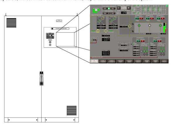
The pumping system can be fully monitored and operated from ICSS through communication link to, and controlled via, the UCP.
