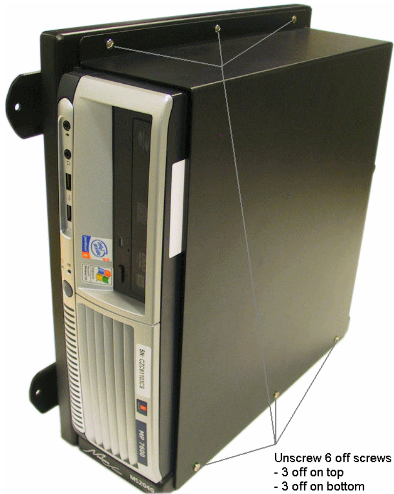
Figure 7 Vertical mounted Damper kit- top
