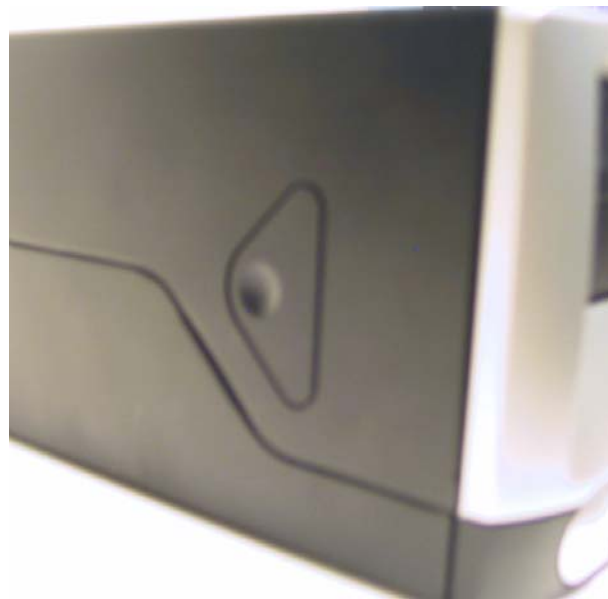
Figure 9 Release lever of the cabinet lid
